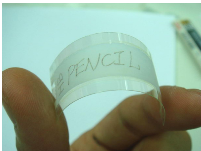
Fig. 4. Image of a bent TiO 2 film compressed at 100 MPa on ITO-PEN substrate with HB pencil writing.
